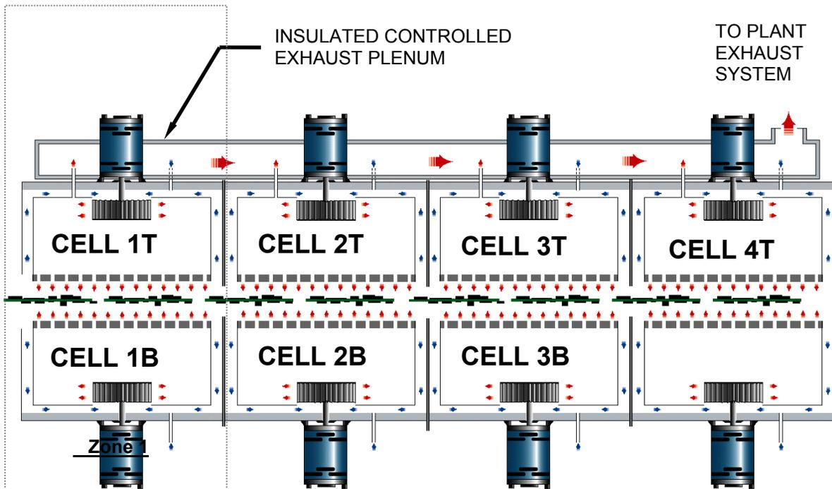
XPM3m OVEN CELL ARRANGEMENT – SIDE-TO-SIDE RECIRCULATION
