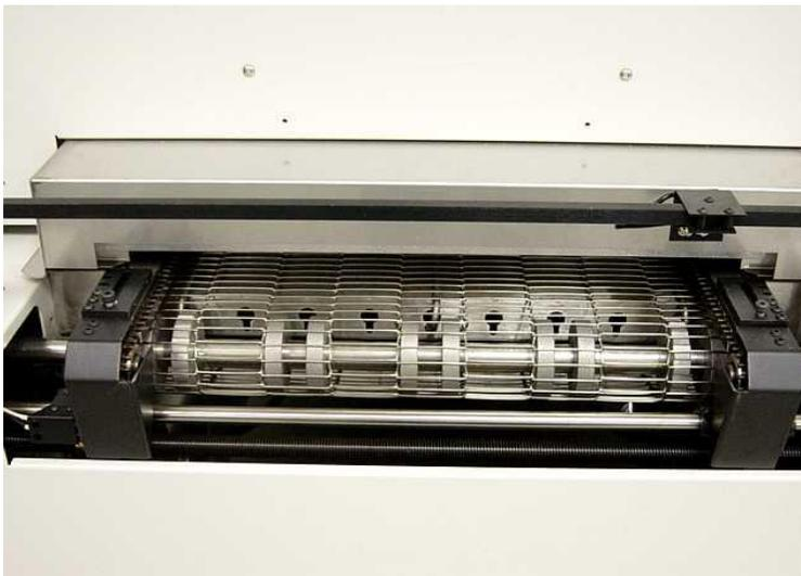
**Approximately 3 inches (76.2mm)** between end of belt and end of rail conveyor (both ends).
