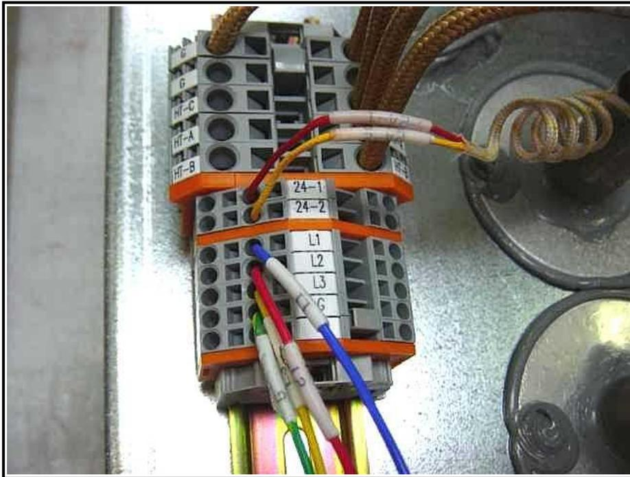
On the back (top / bottom side) of each heater cell is a terminal block assembly.
