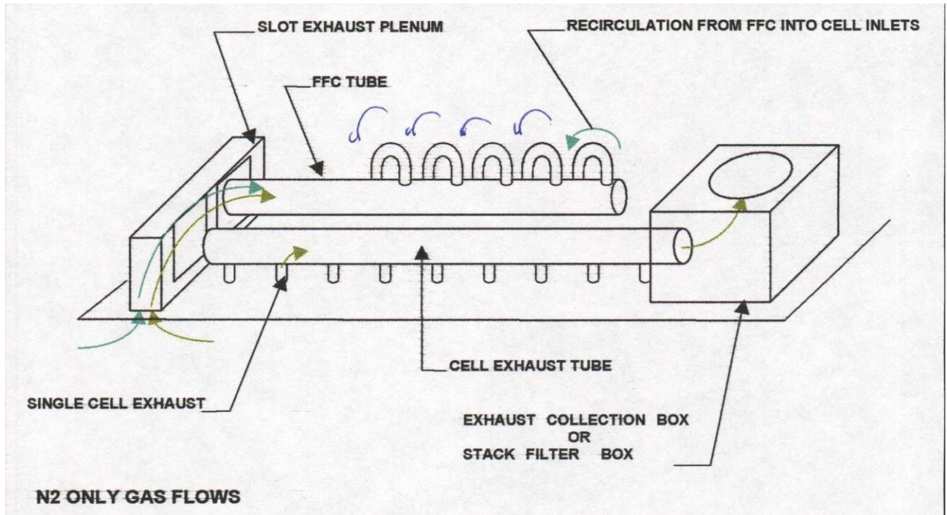
Flow into the controlled exhaust plenum is biased in favor of drawing from the cool zone side. This is accomplished by raising the pressure in the cool zone (by inputting a high percentage of the total oven nitrogen consumption into that area), and by reducing the pressure in the last heated zone (by fully opening the individual cell outlet.) The total oven exhaust is taken from this one port.
