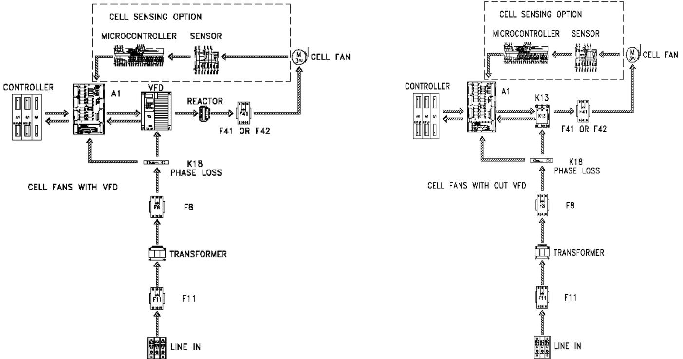
**1) POWER SOURCE:** 3 Phase power is provided to either the line terminals of the Fan Contactor (K13), the primary side of the INVERTER, the 3 phase Fan transformer, or the 3-phase line filter depending on the Oven options and Operating Voltage.
