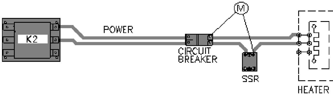
SIMPLIFIED HEATER CONTROL CIRCUIT
