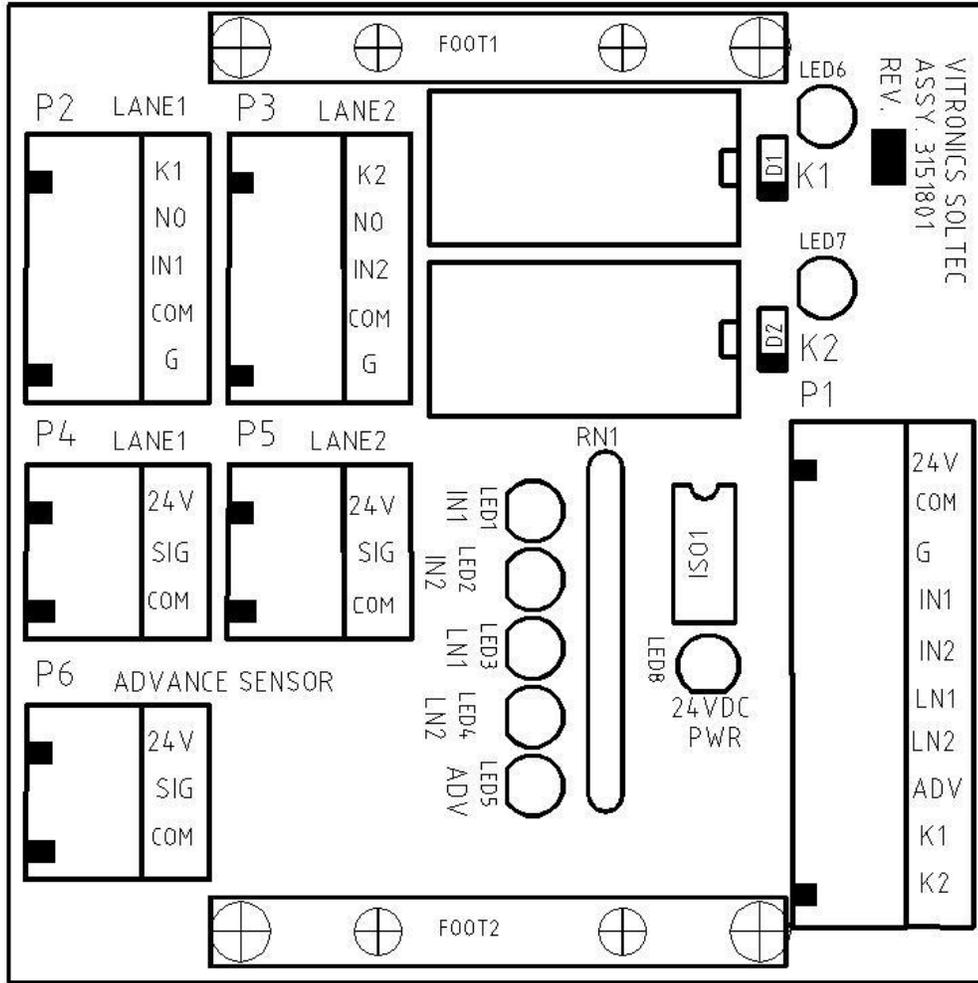
E3151801A ASSY SMEMA/BOARD TRACKING INTERFACE PCB
