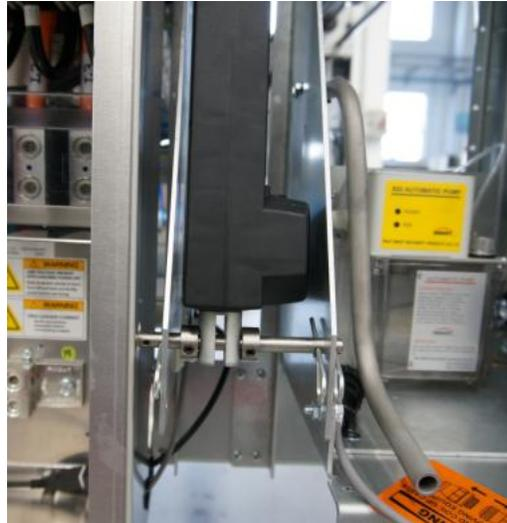
Plug the control cable of the new actuator to the control box. Turn power on to the oven so the actuator can be operated. Perform the actuator set-up and synchronization at this time.
