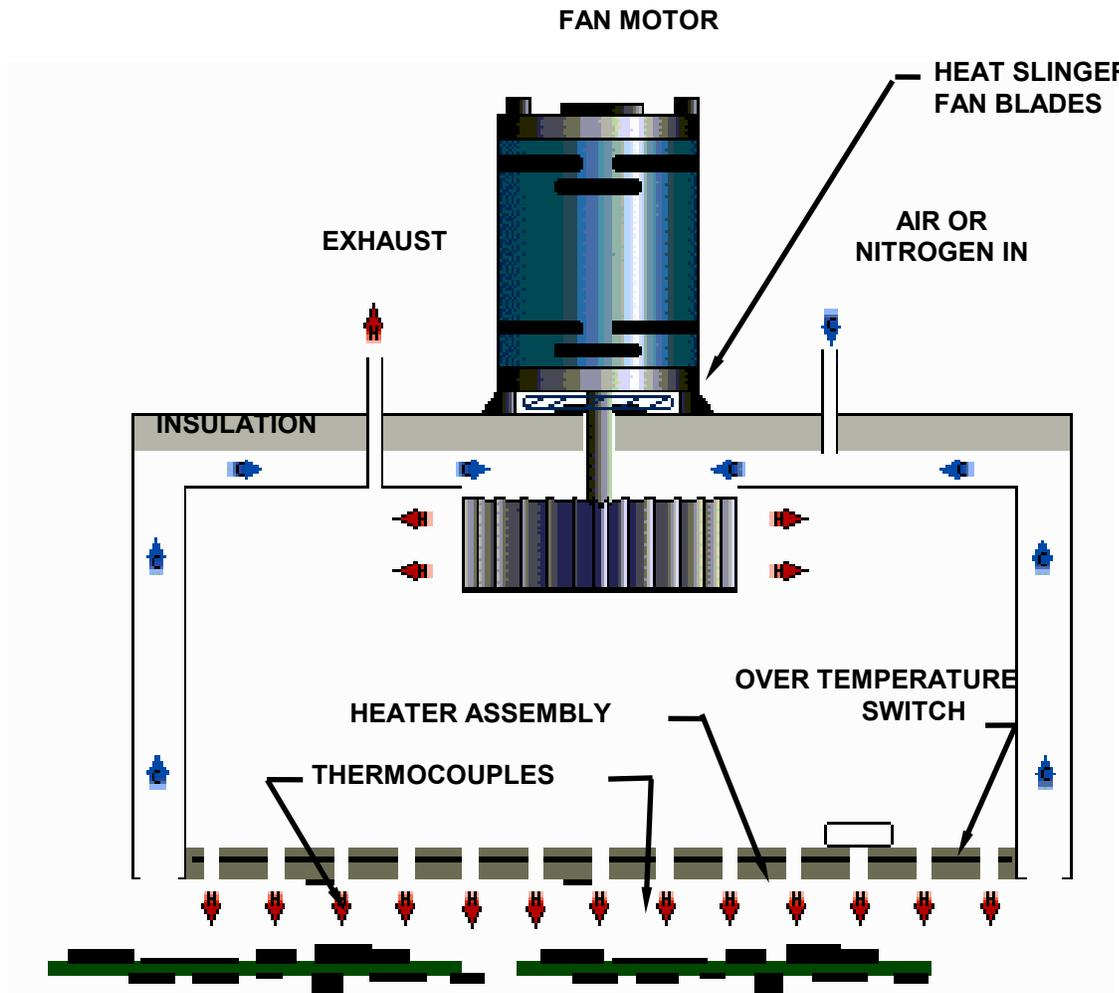
HEATING CELL CROSS-SECTION
