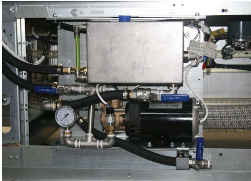
The reservoir is a 1.6 Gallon(6 Liters) stainless steel tank. The level switch in the reservoir monitors coolant level and the flow switch checks return flow. The high-pressure switch trips at 60 PSI. A periodic check of the coolant level in the reservoir is necessary.
