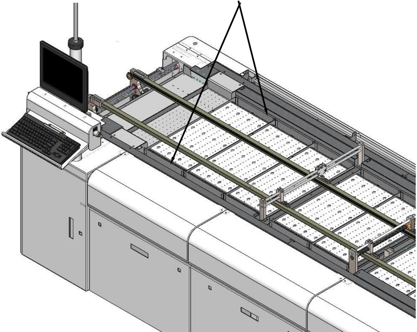
The cells are mounted both above and below the conveyor, as shown, forming a series of “Heat Zones”.
