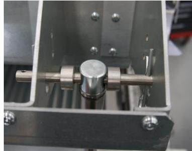
The body of the actuator is accessed through the equipment cabinets on each end of the oven.
