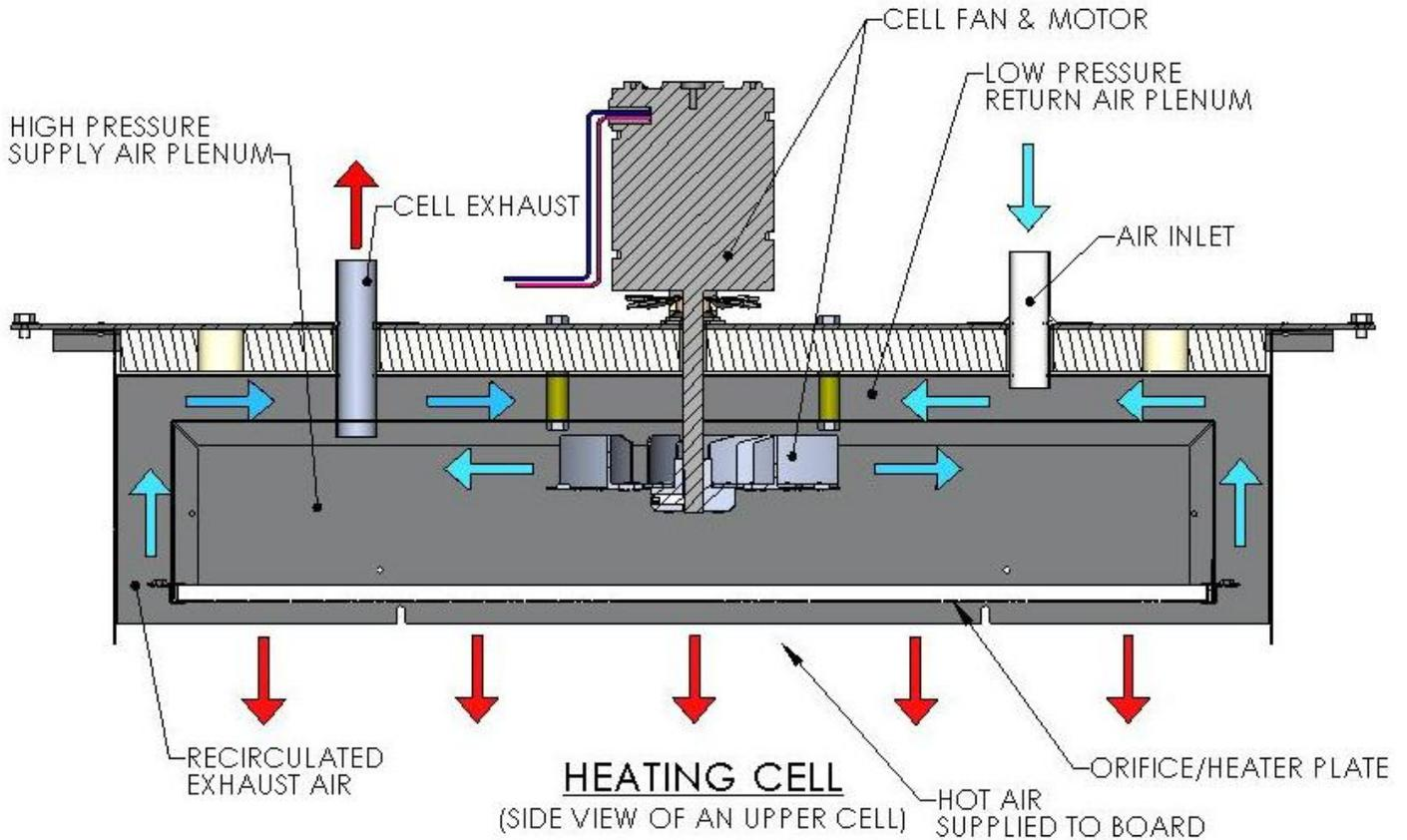
**CONSTRUCTION:** The heat Cells are assembled and sealed as self-contained units with the Fan Motor, and Over Temperature Switch mounted and wired to terminals, and the Thermocouples (1 or 2) mounted and wired to connectors.
