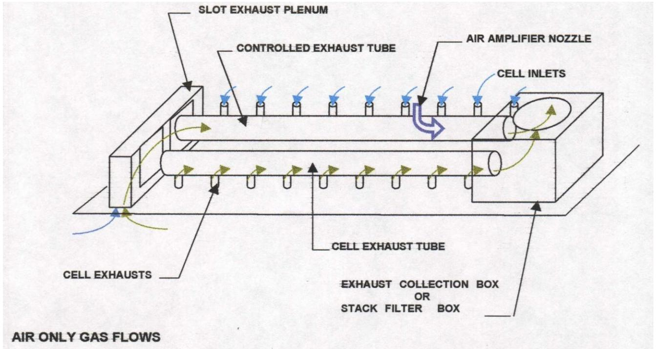
The N2 solenoid and the Compressed Air Solenoid will toggle, following the selection of an Air profile by the operator. All gas flows in the oven remain identical to the N2 Mode, except that Nitrogen is replaced with compressed Air. Flow ratios and all other process parameters remain identical.
