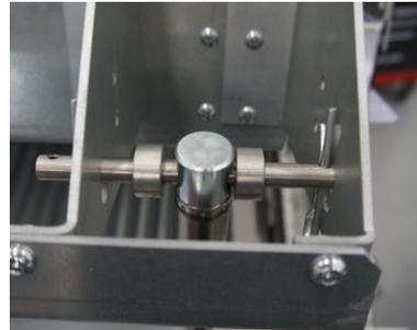
Carefully position the actuator so that the holes for the actuator pivot pin are aligned with the holes in the side of the actuator sheet metal. Insert the actuator pivot pin. As you are pushing the mounting pin into place, install the locking shaft collars on each side of the piston. Replace the two safety clips on the mounting pin. Let the actuator hang from the mounting pin.
