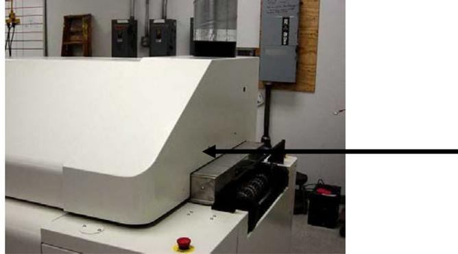
The body of the actuator is accessed through the equipment cabinets on each end of the oven.
